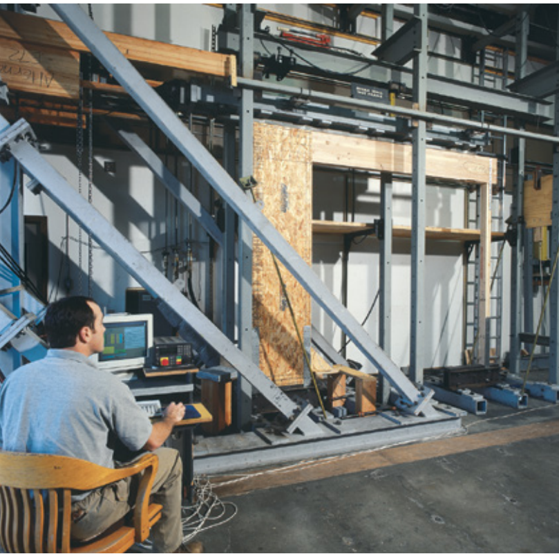
This test in the APA Research Center simulates seismic lateral loads over dozens of cycles to the same wall line. APA researchers can then determine the suitability of various bracing details for seismic performance, such as extending the glulam header over the narrow end wall.
